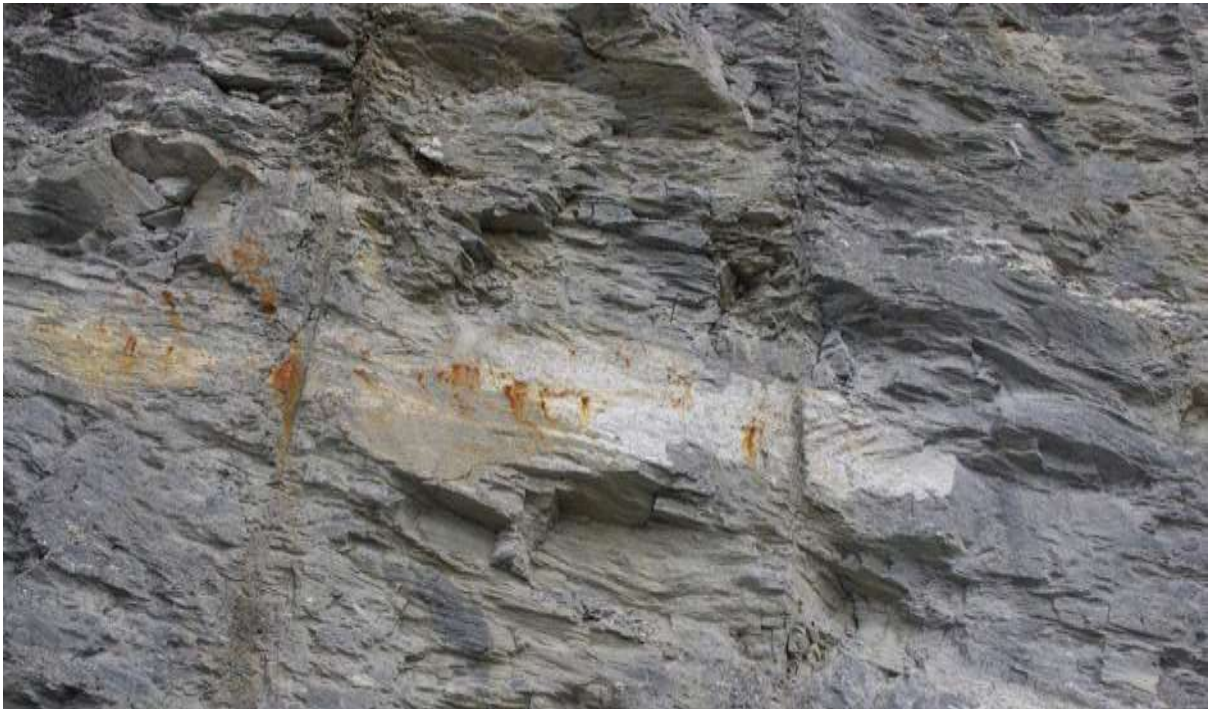
Plate 5.13 mixed bedding planes (KE, DG, with calcite banding central section of the quarry face
